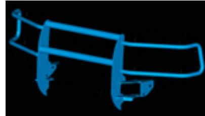
WARN engineers utilize computer-aided design programs to insure the WARN Trans4mer mounting kit with a WARN winch fits the specific make and model of your vehicle.
