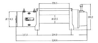
534.4 mm L. x 160 mm D. x 193.2 mm H. Mounting Bolt Pattern: 254 mm x 114.3 mm
